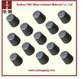
Grinding cylpebs are widely used in cement, mining and chemical industry etc.. The hardness reaches up to 64HRC(the surface and inner hardness tolerance with in 2HRC), which makes the high wear-resisting property. In addition, the distribution of the hardness gradient is average. The property- low wear rate, good toughness, prolongs its life, improves the productivity of the ball mill, and lowers user's cost. Our quality is accord with GBT17445-2009 China national standard.
